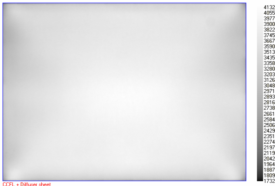
Figure 5: Image of the CCFL backlight of figure 1 with the diffuser sheet.
